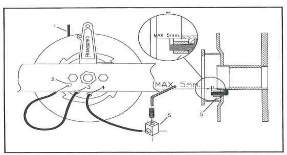
Drawing "B" Attaching cable to wire drum
